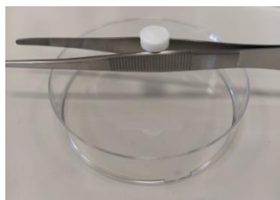
Fig. 1. Photo of the fabricated porous galactose hydrogel form.
